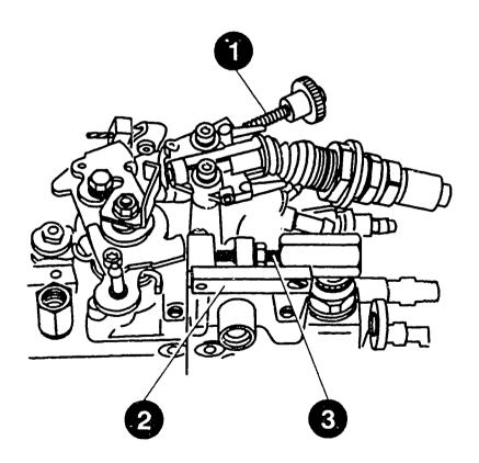
Position speed-control lever by way of knurled screw (arrow) at spacer.
